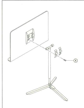
9. Attach the desk assembly (1) to the T-tube, using the pivot brackets (3) and screws (4).
