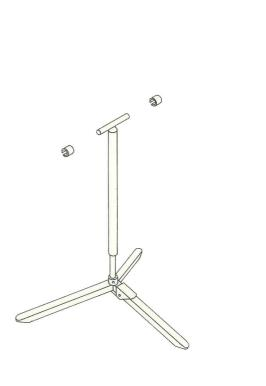
8. Slide the friction pivots (2) over the T-tube.
