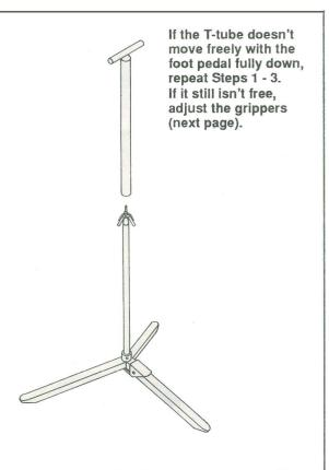
5. Fully depress the foot pedal and slide the T-tube (5) over the inner tube. With the pedal fully down, the T-tube should move up and down freely. If the T-tube slides down too easily with the pedal released, adjust the grippers (next page).
